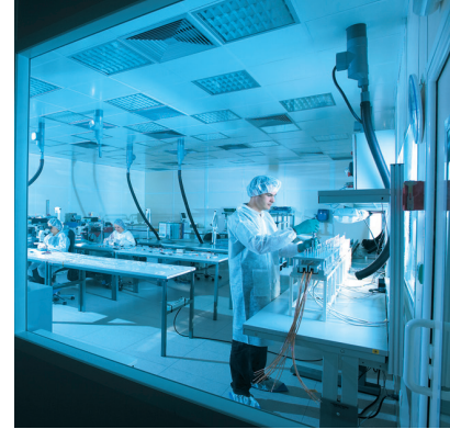
CLASS 100000 CLEAN ROOM
