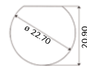
PANEL CUT OUT
