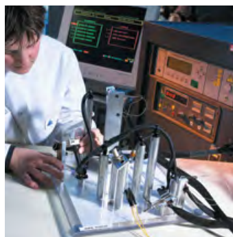
▲ AUTOMATIC CONTINUITY & INSULATION RESISTANCE TEST
