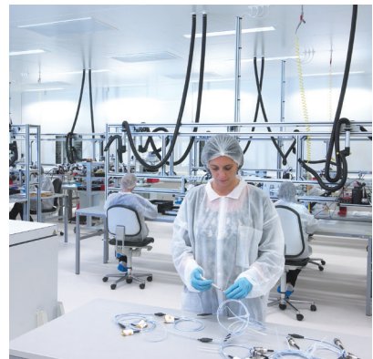
MANUFACTURE OF HARNESSSES IN ISO 8 CLEAN ROOM
